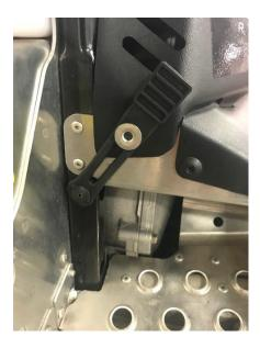
Right front lower, use stock screw hole for stud/peg mount, locate strap position relative to picture, use same process as previous to install.
