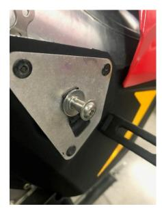
Lower rear both sides, install flange head screw with washer thru stock hole, install washer, Blue Loctite and t-nut then tighten securely. Locate strap relative to picture, drill 3/16" hole and rivet strap in place.
